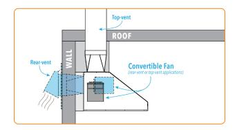
Power Vent Hoods are for outdoor use only and must be wall mounted. See owner's manual for detailed installation instructions and additional information.
